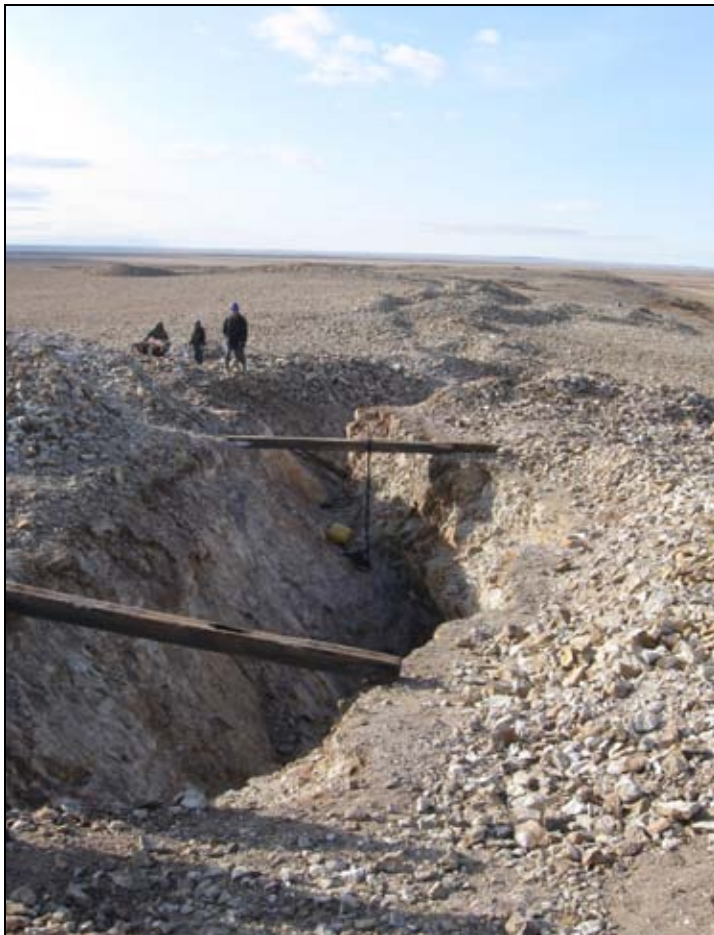
Figure 1.3 Pilot mining of fluorspar at Dai-Uul. Under the exploration licence the company can extract 400t of mineralisation. Miners extract high grade vein type mineralisation using compressor driven jack hammers, buckets and winches. The vein dips about 55° to the west (photo looking S).
